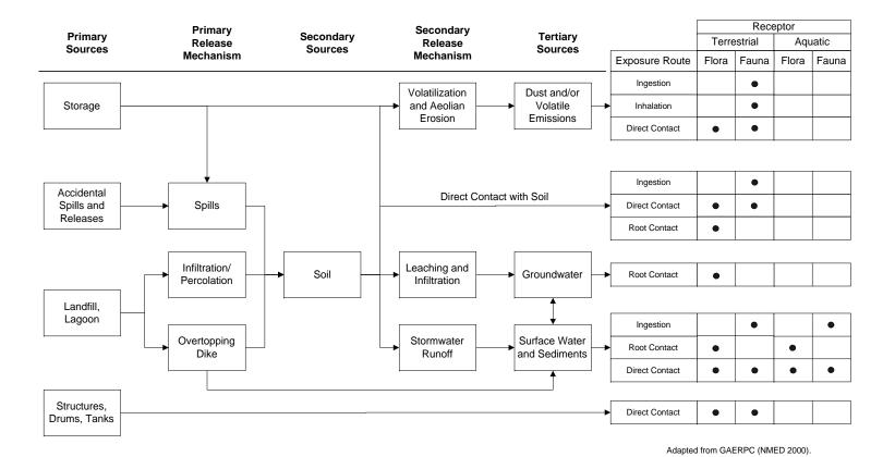
Figure 2. Example Preliminary Conceptual Site Exposure Model Diagram for a Hypothetical Site
