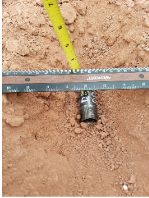
Seed DGM-001 buried north-south horizontal at a depth of 4"
