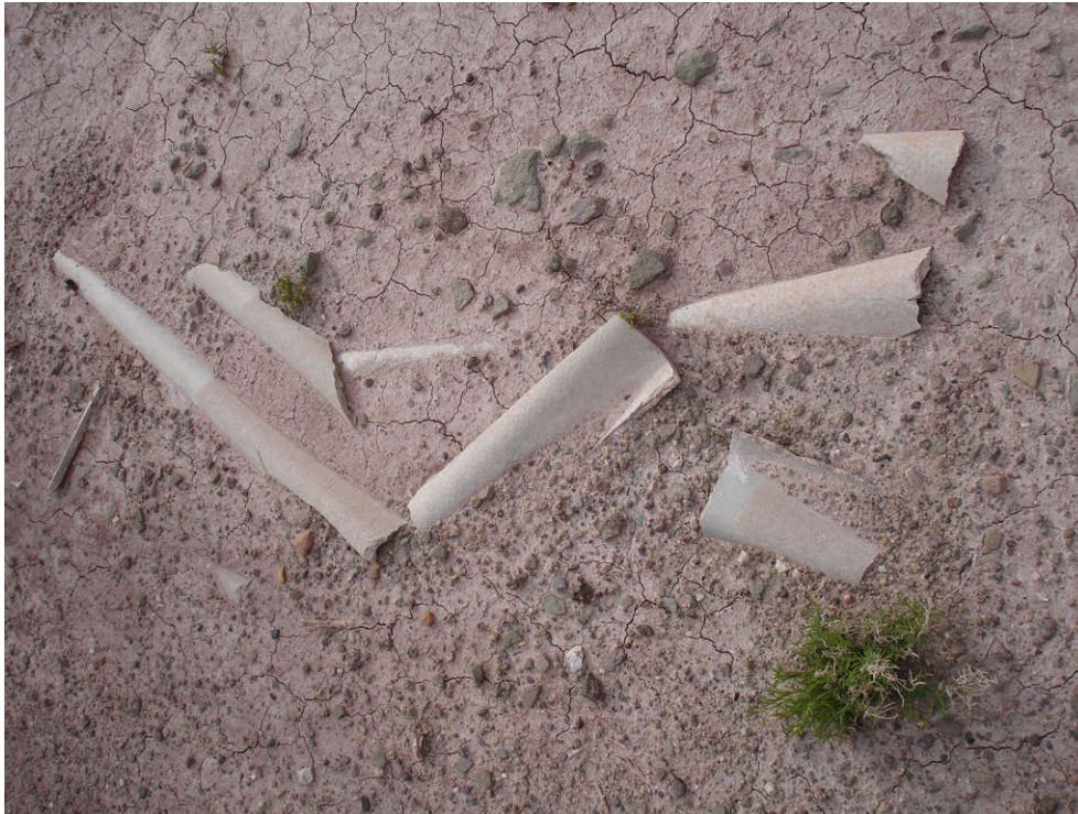
Photo 5-7: AOC 69, showing potential ACM roof tile.
