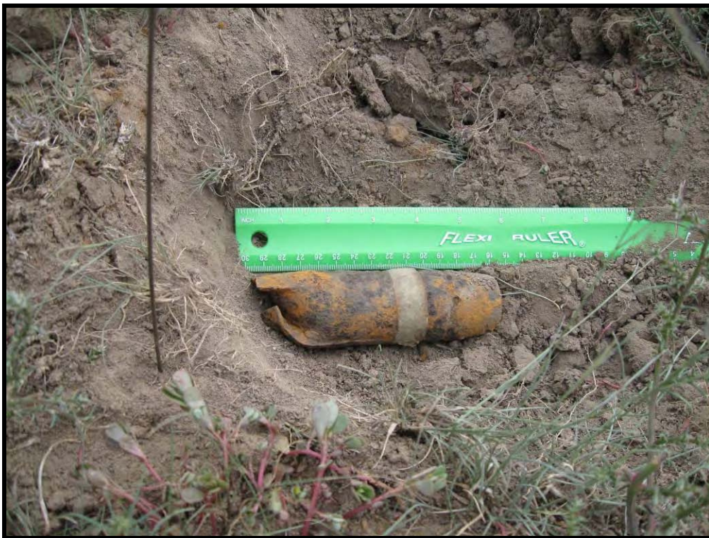
Burnt Out 57-mm Projectile/Munitions Debris
