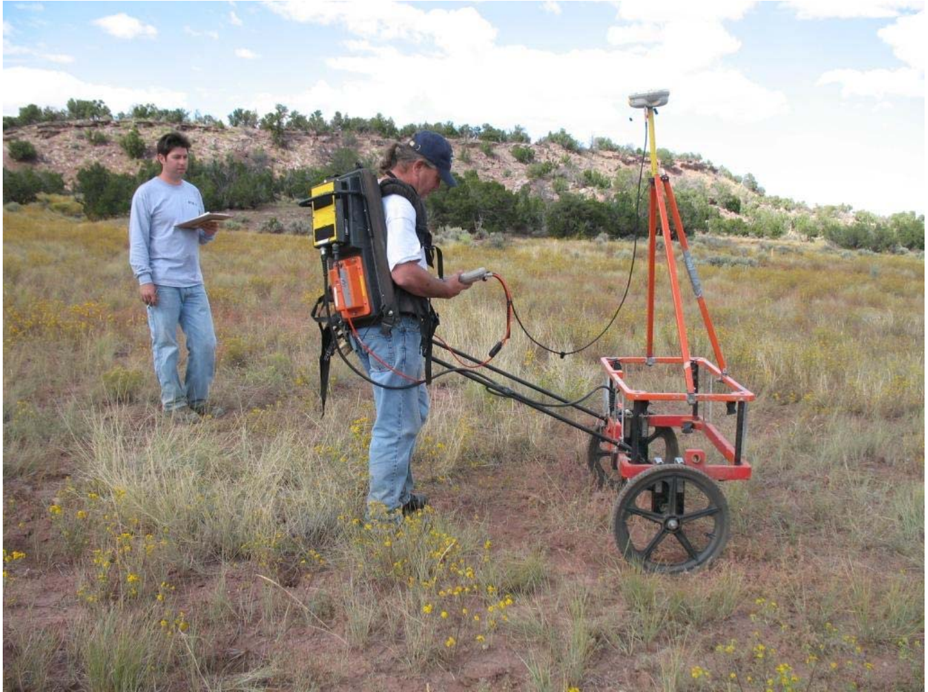
Figure 4-1. EM61-MK2 Metal Detector
