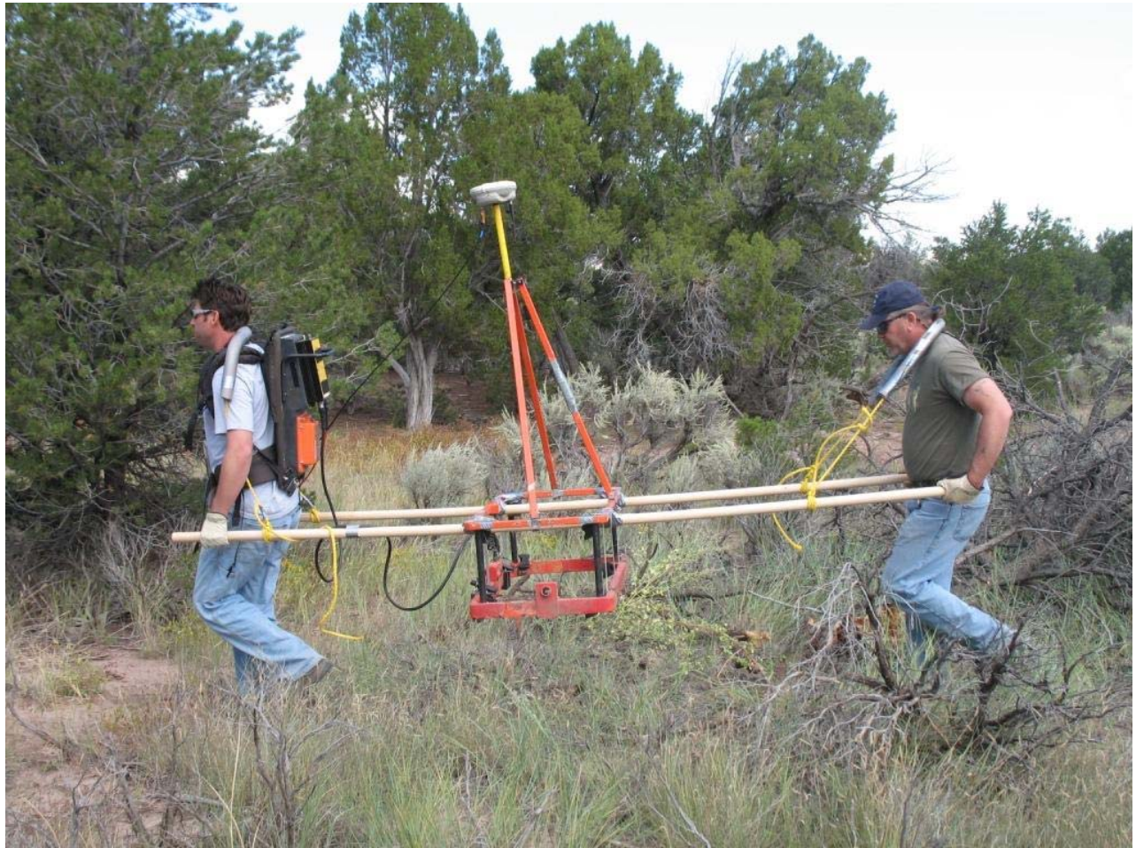
Figure 4-3. EM61-MK2 Metal Detector in Litter Mode
