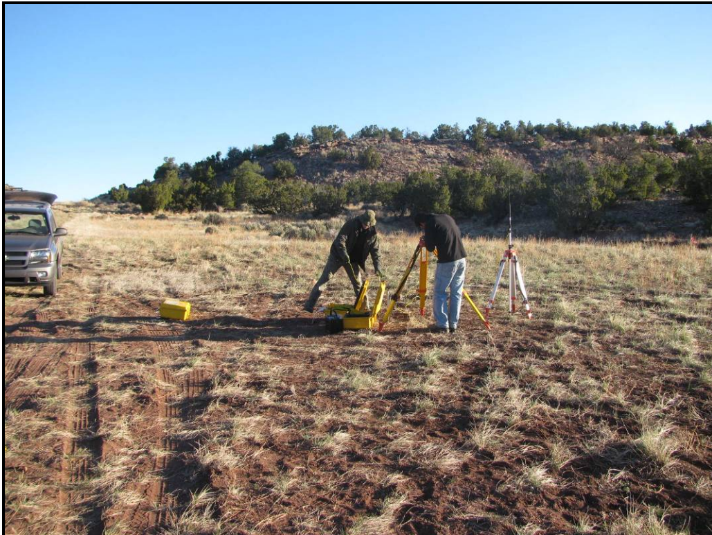
Setting Up Tripod/Base Station for EM-61 Operations
