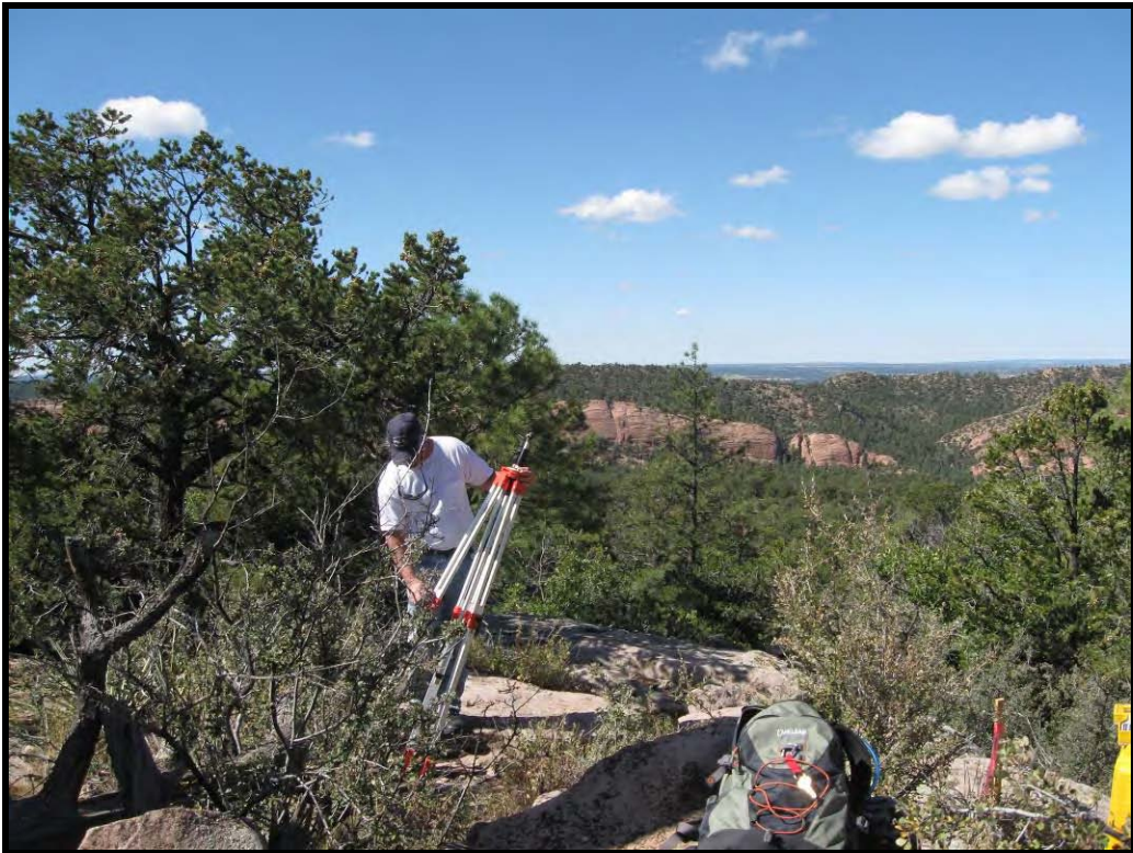
Setting Up GPS Base Station for QC Operations
