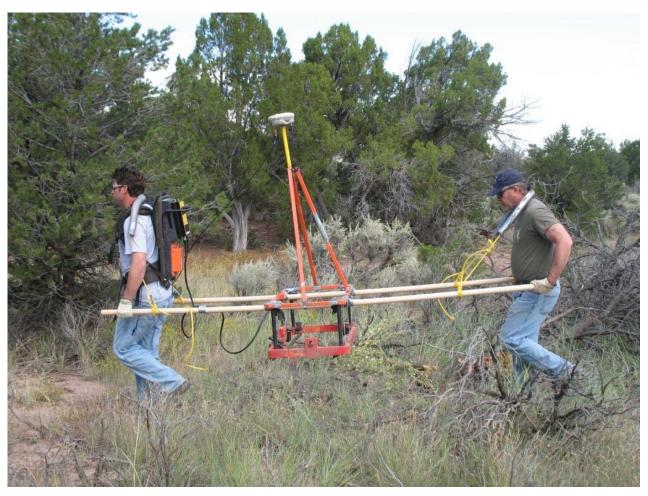
Figure 4-3 EM61-MK2 Metal Detector in Litter Mode
