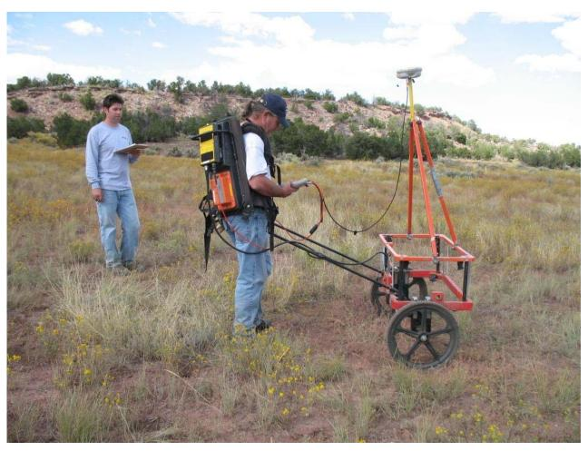
Figure 4-1 EM61-MK2 Metal Detector
