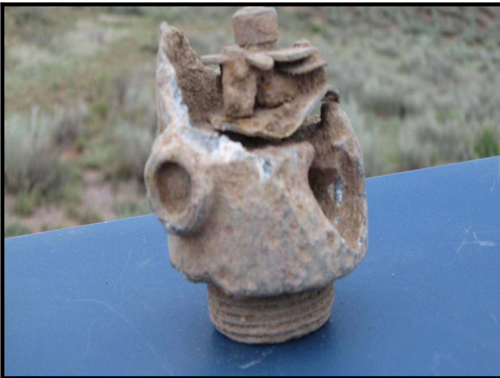
Close Up of Damaged M-120 Fuse
